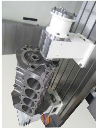
Automatic 4th Axis Block Roll Over Fixture
