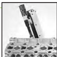
Pneumatic Head: Adjustable to 25° in either direction for cant valves
